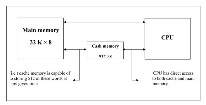
This cache memory block is the only block that communicates directly with the CPU at high speed. The fundamental idea of cache memory is that by transferring the most frequently the access program instruction and data from the slower, cheaper internal memory to the expensive fast cache memory when they are needed by the CPU.
