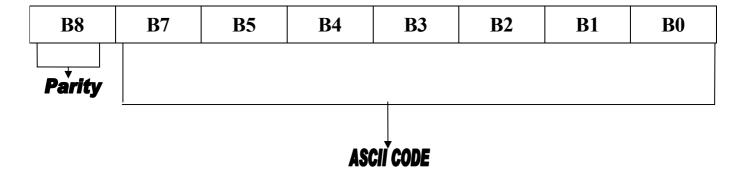
(The 8-bits ASCII code with parity)
