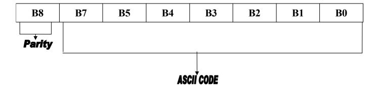
(The 8-bits ASCII code with parity)
