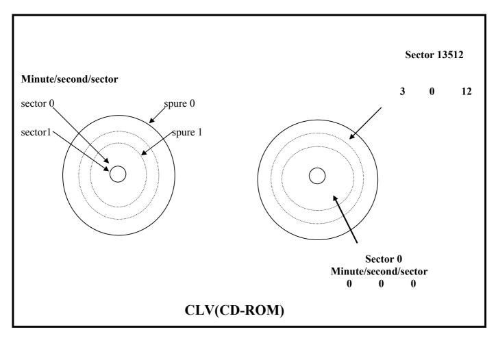
Therefore, the rotation speed of the drive increases as the head moves from the inner edge of the medium to it outer edge. This one of the reasons why a CD-ROM drive has significantly slower access times than a hard drive. It must constantly change its rotation speed. The time to speed up and to slow down becomes significant. Also, it's much more difficult to find
