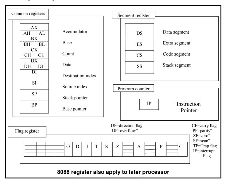
The different register assignments are designed to duplicate the way in which a program processes data, which is the basic task of a microprocessor.
